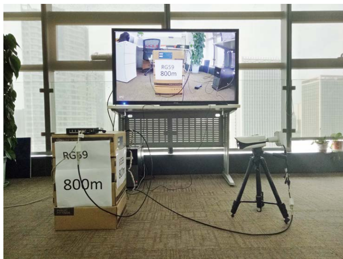
Test of 800m transmission over RG59 cable
