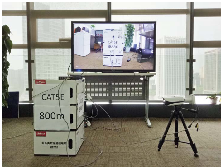
Test of 800m transmission over Cat5E cable
